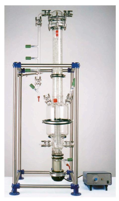
Pict. 1 Laboratory unit for the absorption of reaction gases
